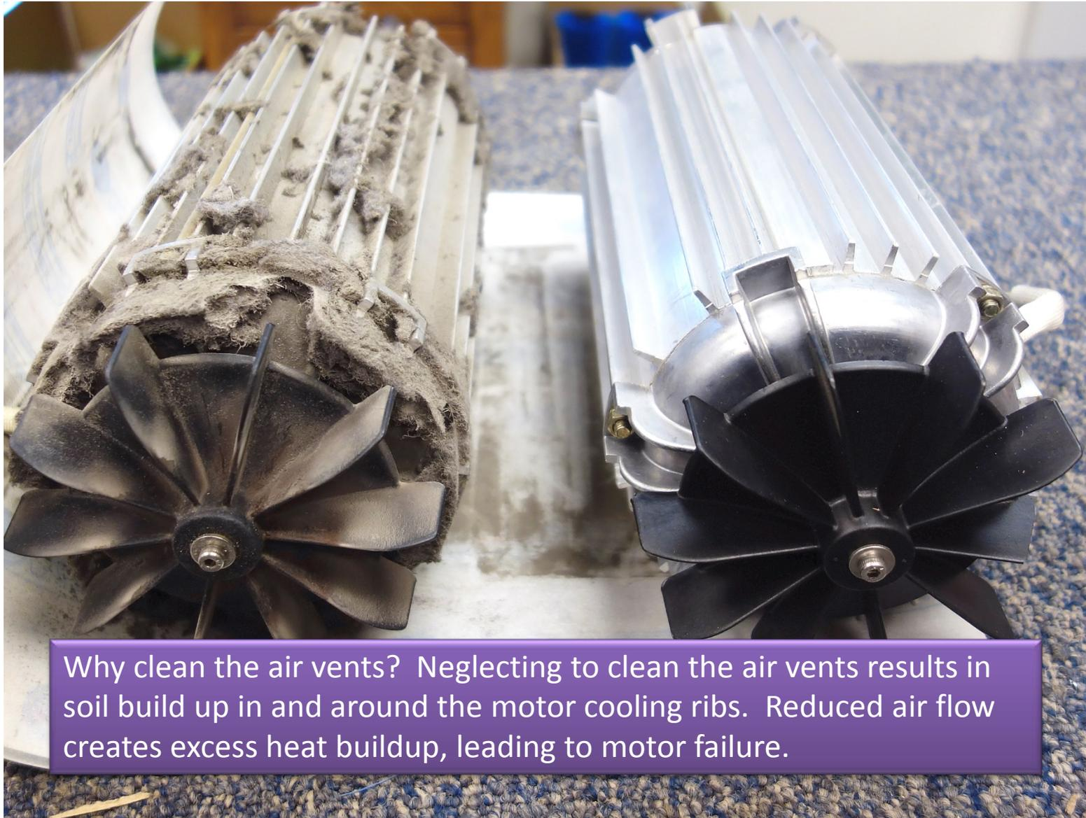
Why clean the air vents? Neglecting to clean the air vents results in soil build up in and around the motor cooling ribs. Reduced air flow creates excess heat buildup, leading to motor failure.
