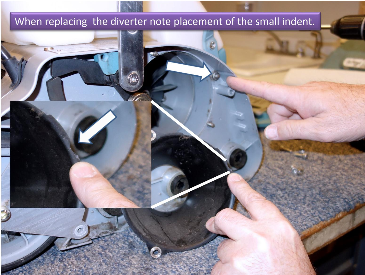
Vacuum inside of side cover assembly. Remove all loose soil.
