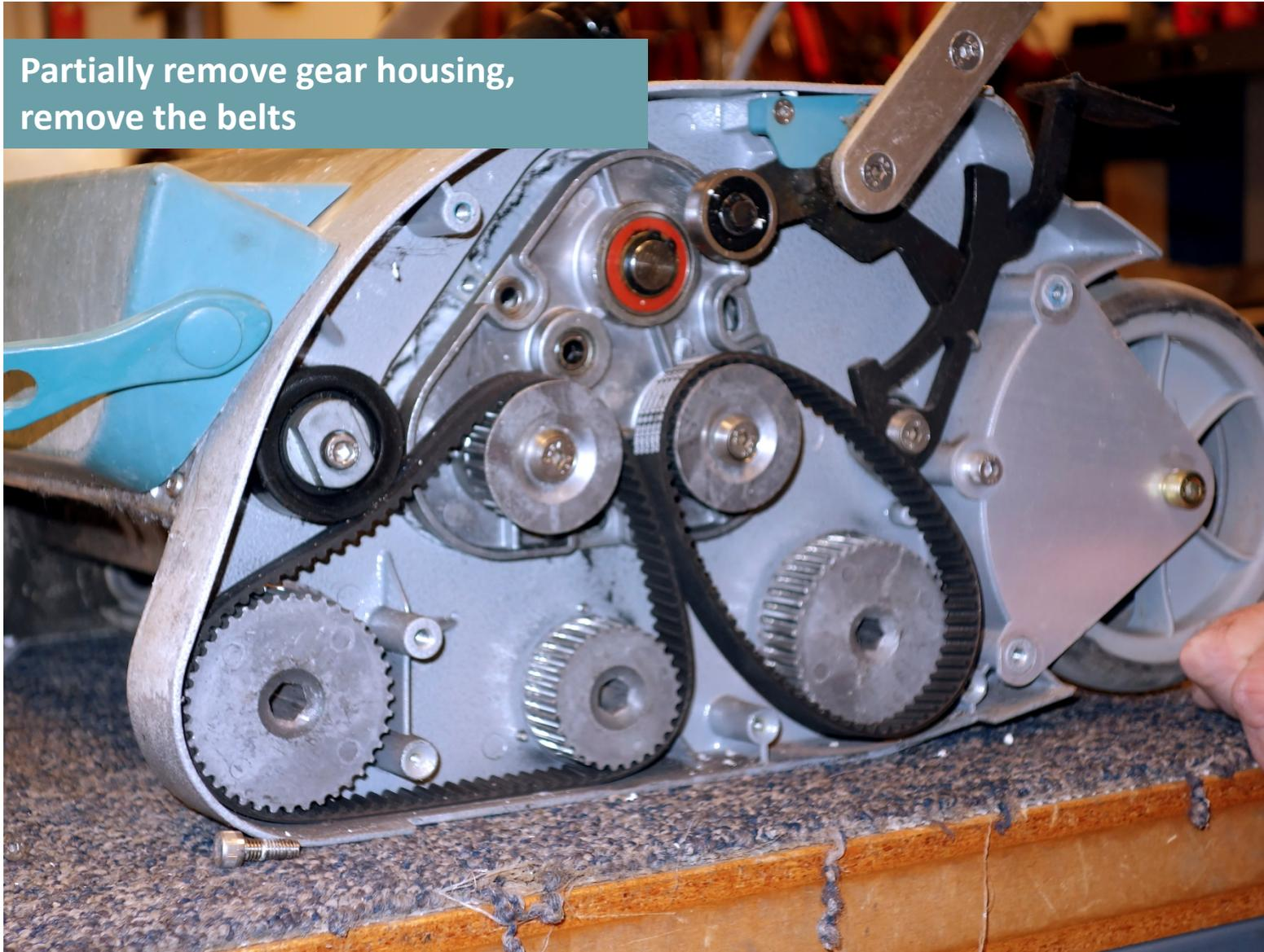
Remove gear housing from side housing assembly. Note stripped gears!
