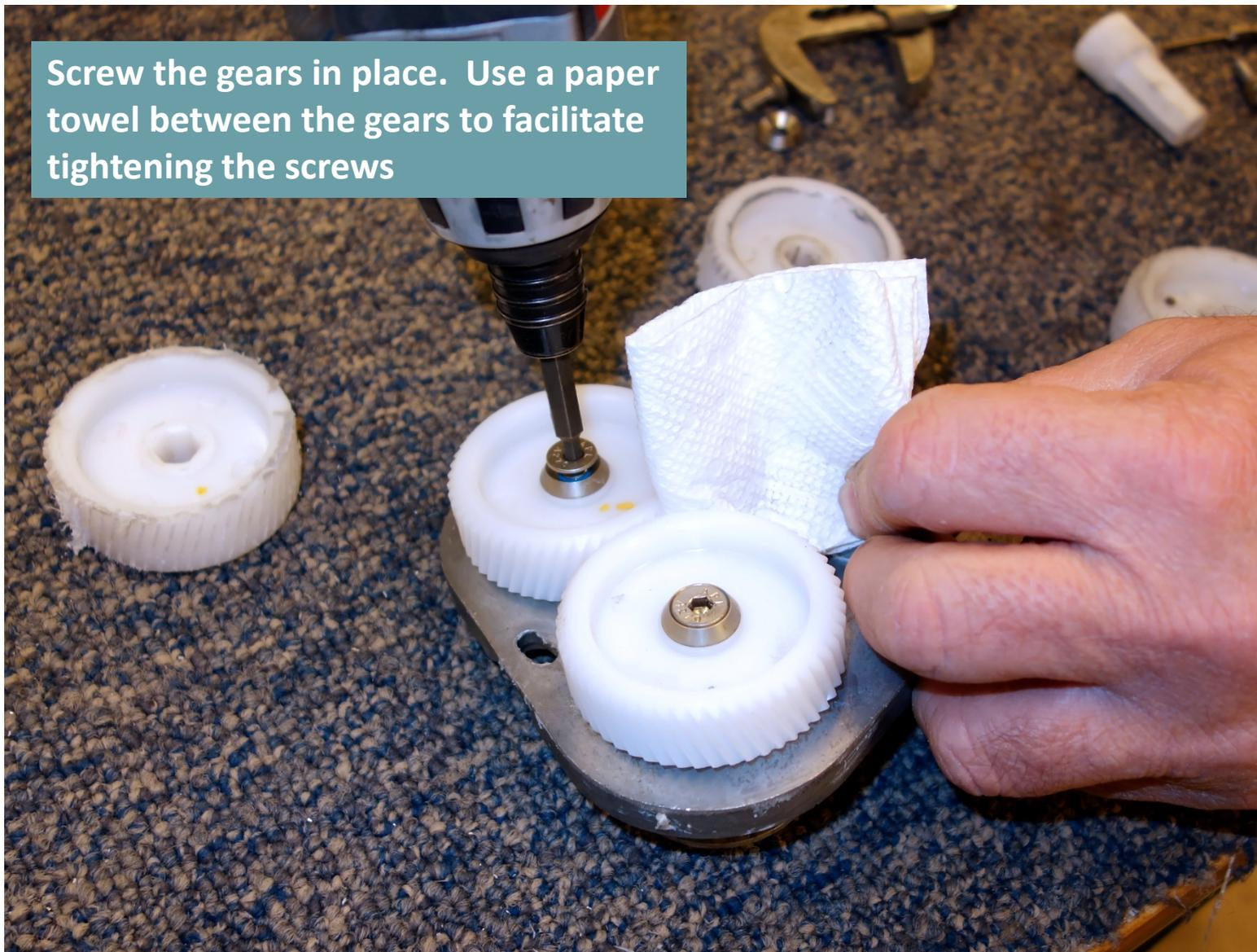
Please note there are 2 Yellow dot right hand gears and 1 Blue dot left hand gear. The orientation is shown below. The gear housing fits into drive housing only one way, as shown.
