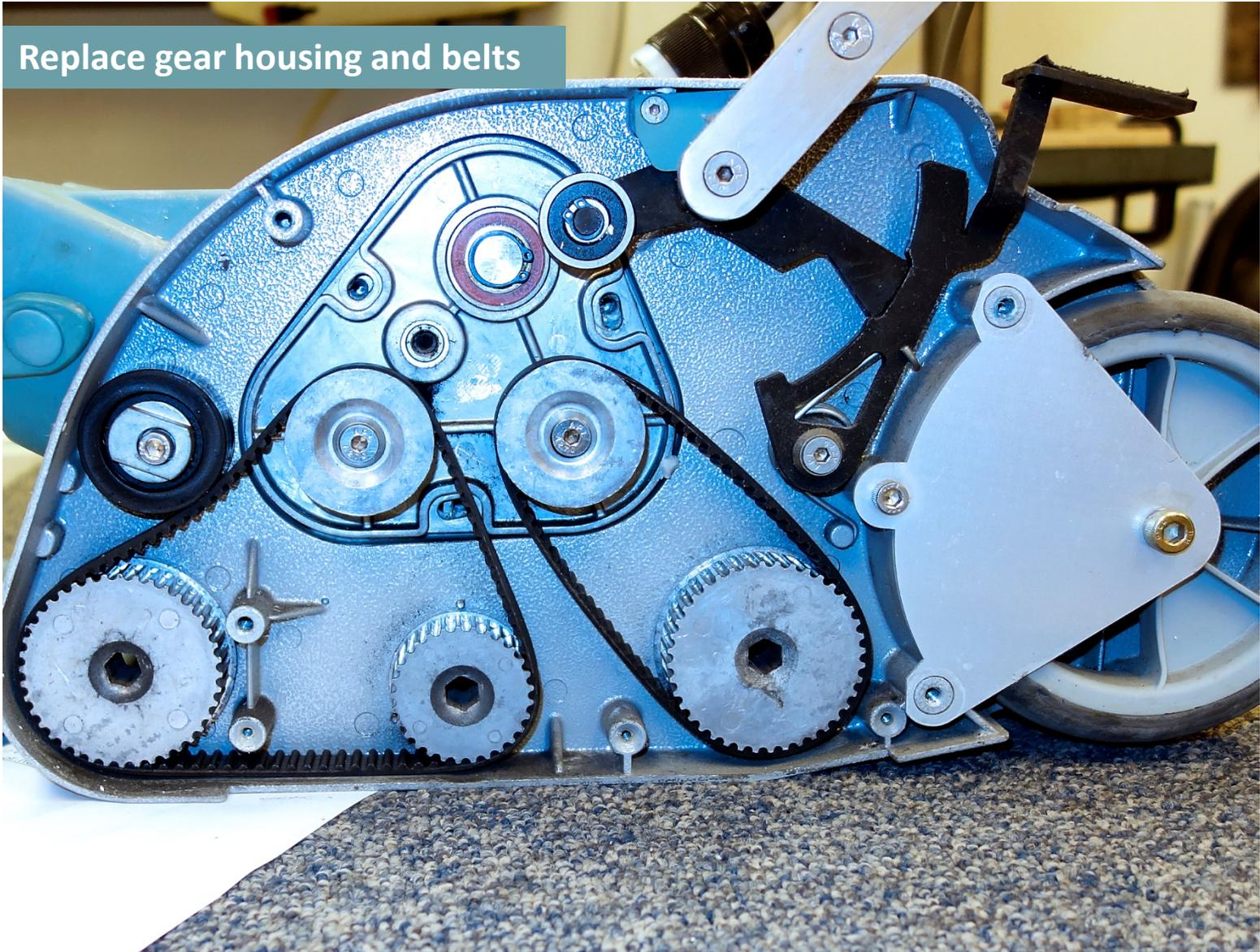
Replace the 3 screws then use a screwdriver to lift gear housing to tighten belt as shown. Then tighten screws while still lifting with screwdriver
