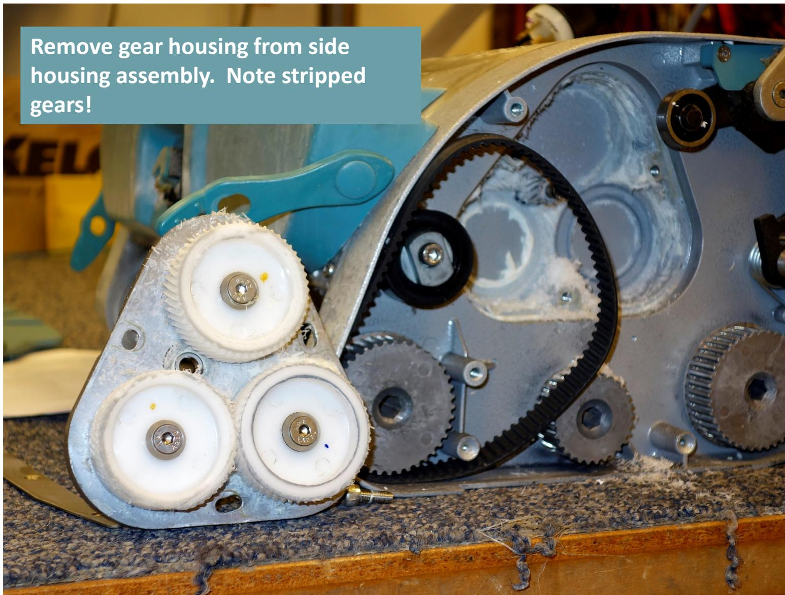
Remove damaged gear(s)
